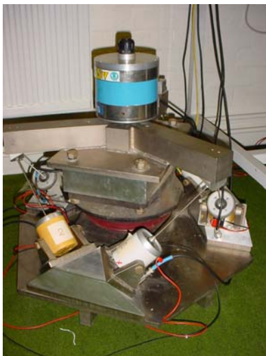
Fig. 2: Experimental active mount
