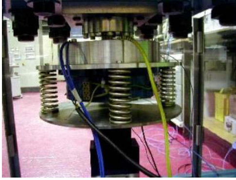
Figure 1: Prototype Actuator for a “Smart Spring” Mounting System
